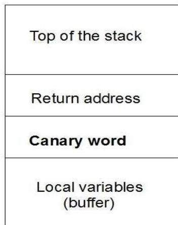
Fig. 3. Use of a canary word for buffer overflows protection.
