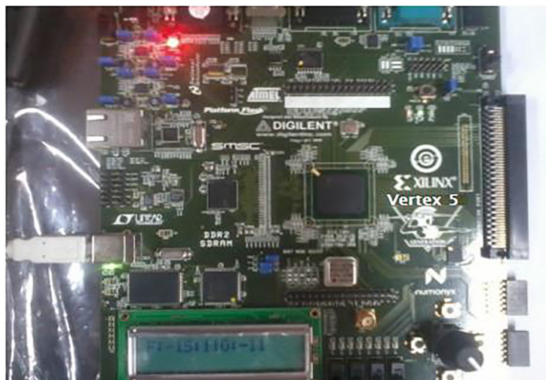
Fig. 5. FPGA implementation of Baugh-Wooley Multiplier in Vertex 5 kit
