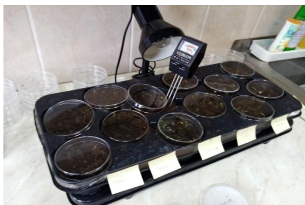
Figure 9: Using a sensor to monitor soil pH and moisture
