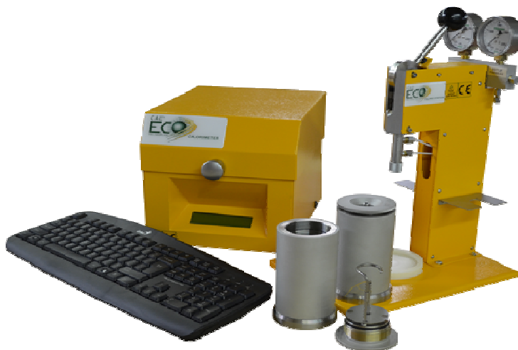
4. Figure: The bomb calorimeter apparatus
