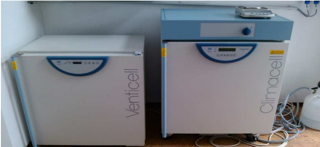
5. Figure: The Venticell 111, Climacell 111 equipments and the milligram preciseness balance.
