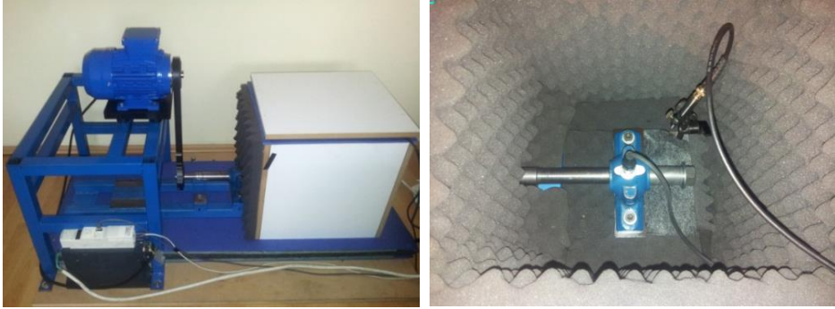
Figure 19. Bearing test rig (left) test bearing in acoustic chamber with pyramidal RAM and electric microphone (right)
