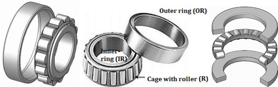
Figure 2. Roller bearings: cylinder (left), tapered (middle), thrust (right)
