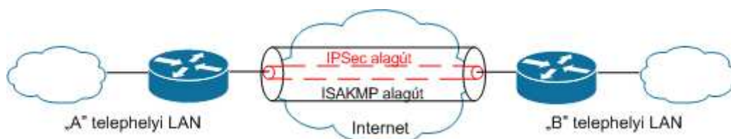
8. ábra: IPsec Lan-to-Lan VPN
