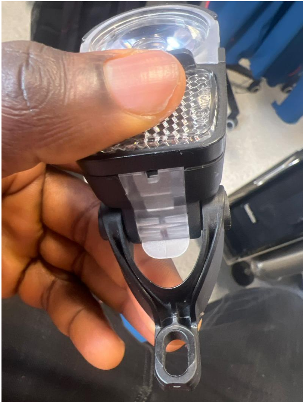
High stress concentration at the neck region of the Folk bracket (reason for failure)
