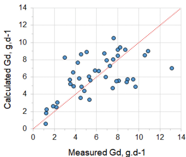
Fig. 4. Scatterplot of the measured and calculated daily amount of anthropogenic gadolinium released to the wastewater treatment plant.
