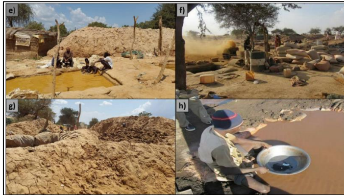
Figure 4-32. Gold extraction practices in ASM areas (a: miners around a small artificial pool filled with water for ore washing and panning; b: breaking rocks generates dust clouds; c: improper waste disposal; d: manual amalgamation of gold using mercury in a pan filled with muddy water).
