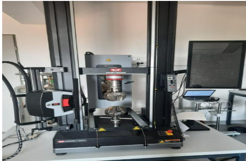
Figure 25: Instron 6800 for tensile strength experiment
