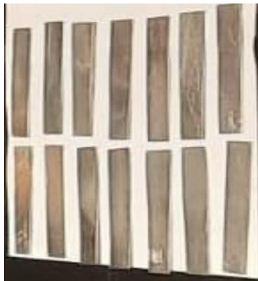
Figure 30: Unclean surface of the adherends after cutting
