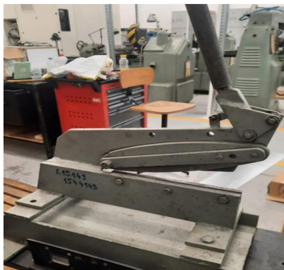
Figure 28: Cutting of adherends from alloy by the manual sheet cutting tool
