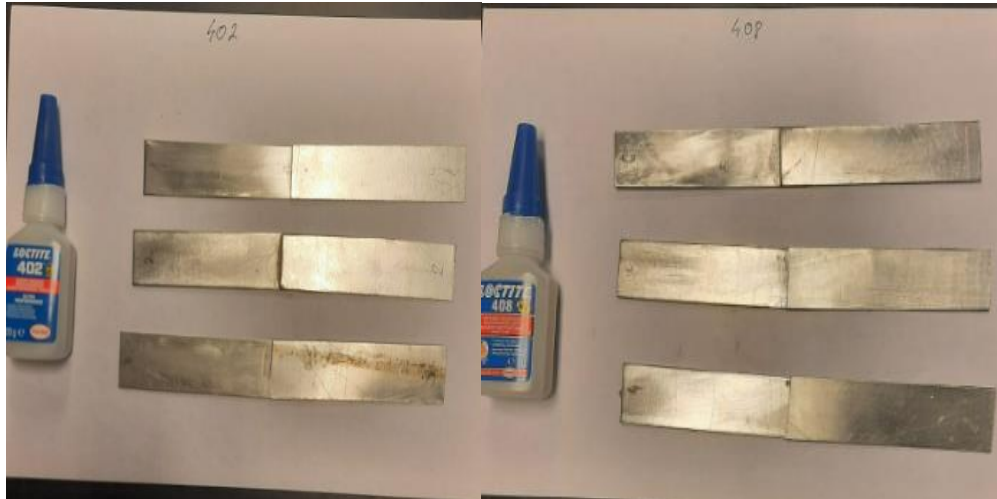
Figure 34: Application of Loctite 402 and 408 for bonding.
