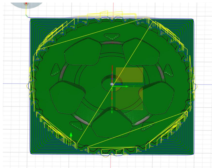
Figure 3.9 The path for processing the teeth of the sprocket
