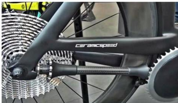
Figure 1.13 Bicycle Shaft Drive Transmission System[27]
