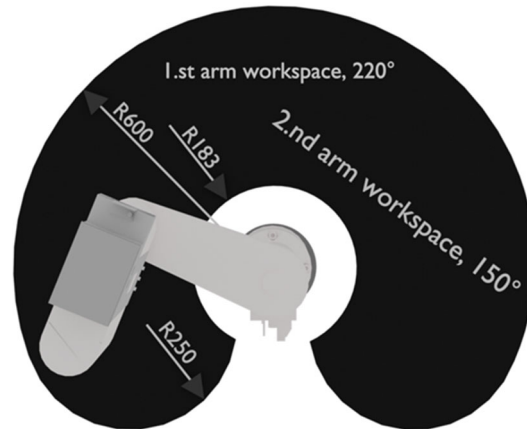
Figure 2. The workspace and the corresponding values of robot arms degrees of SCARA robot unit.
