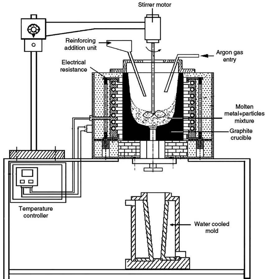
Fig. 1. Schematic diagram of experimental set-up for manufacturing AA2024/B<sub>4</sub>Cp composites [11]. Re-published under CC BY 4.0, without any changes
