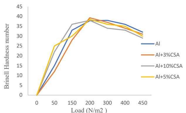
Fig. 3. Brinell hardness number vs load N/m<sup>2</sup>
