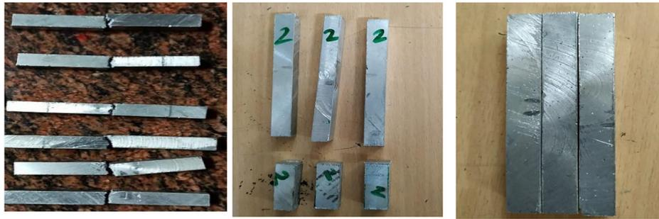
Fig. 5. Observation of Charpy test
