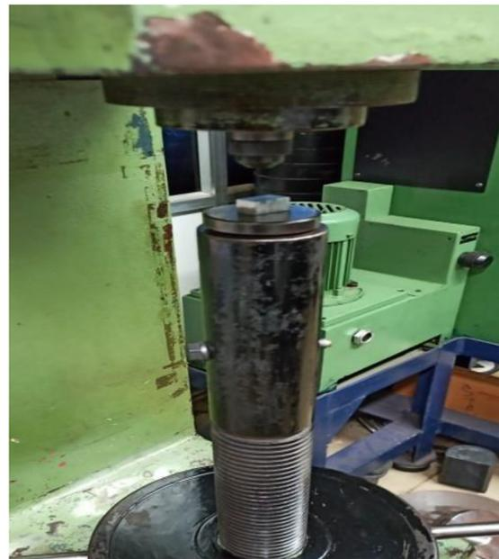
Fig. 2. The Brinell Hardness Test setup
