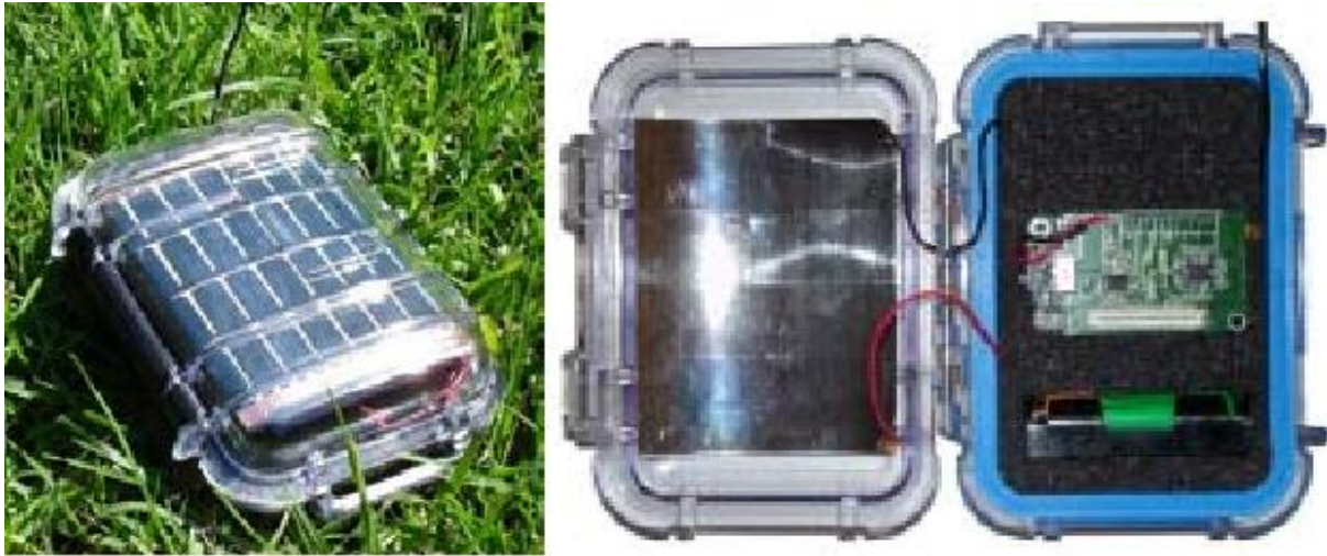
Figure 3.3: Heliomote: an energy harvesting sensor node, which provides environmental energy tracking capabilities [77]
