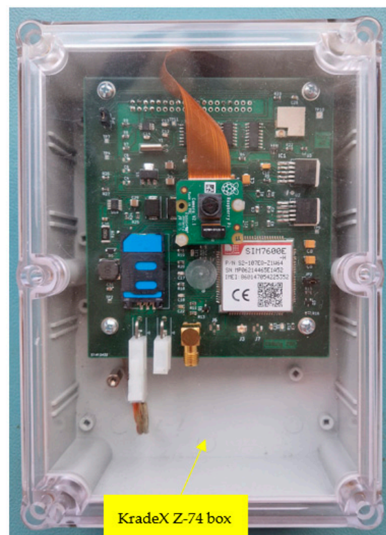
Figure 8. Sensing device case with transparent cover. The battery is placed behind the printed circuit board (not visible).
