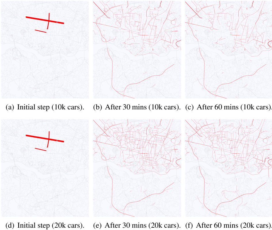
Figure 4.12: The change of the distribution of cars during the simulation (10,000 and 20,000 cars). The thickness of the street is proportionate with the number of cars on the street. Source: [9].
