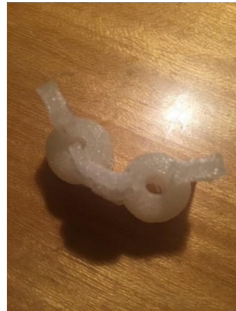
Figure 15: MK.1 XP1 original print design with full bridge and clamp
