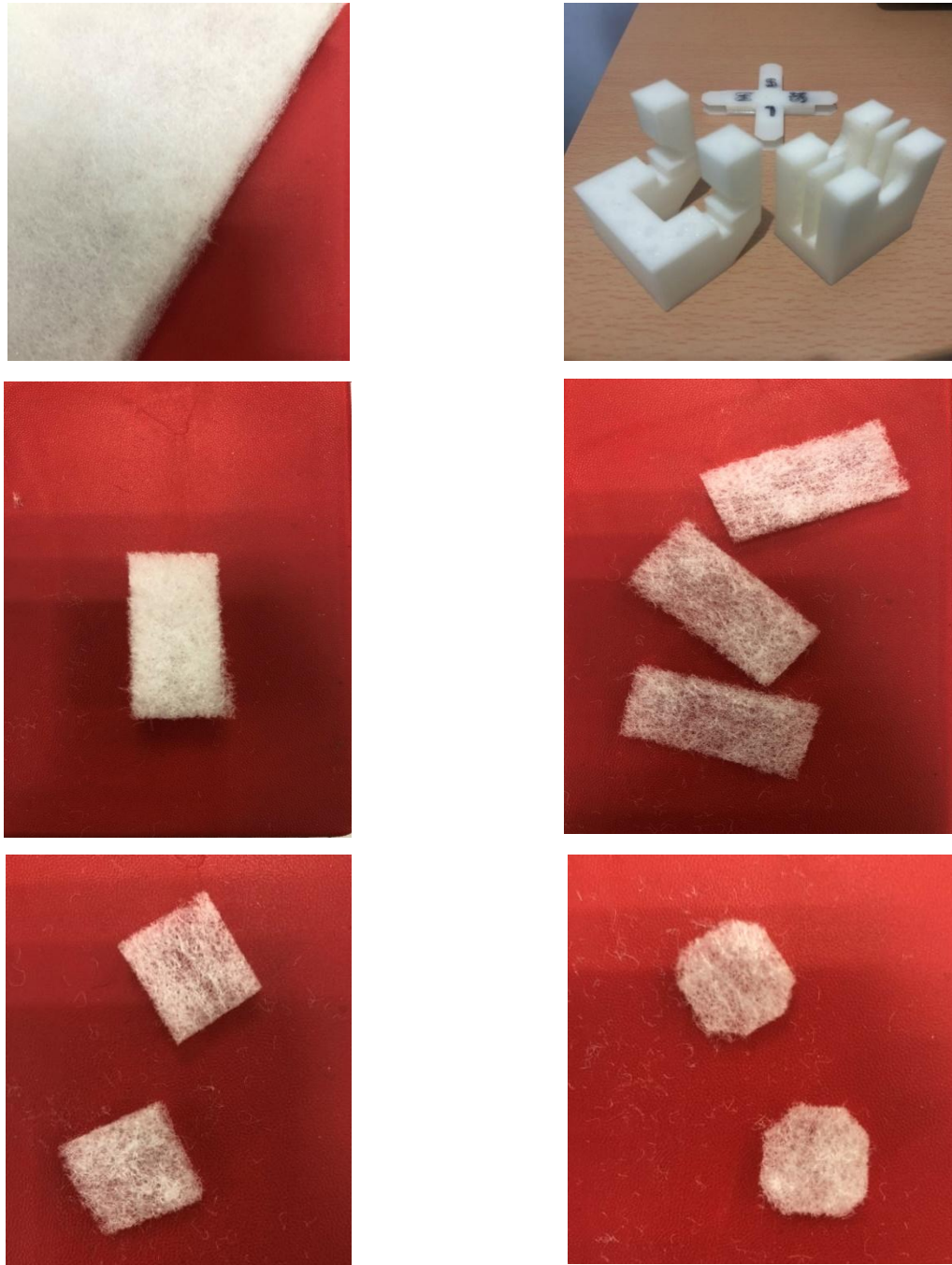
Figure 36: Preparation steps of an appropriate size filters
