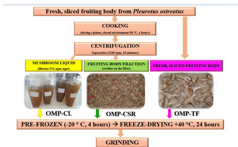
Figure 1. The schematic figure for the manufacturing process of mushroom powders. Freeze-dried oyster mushroom powder from cooked mushroom liquid-filtrate (OMP-CL); Freeze-dried oyster mushroom powder from the cooked fruiting body: residue on the filter (OMP-CSR). Freeze-dried oyster mushroom powder from the total fresh fruiting body (OMP-TF).
