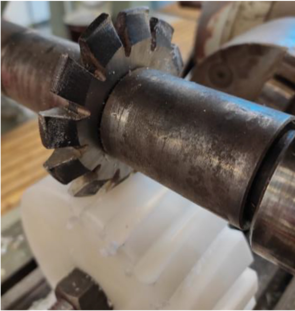
Fig. 10. The geometry of the module disc milling cutter
