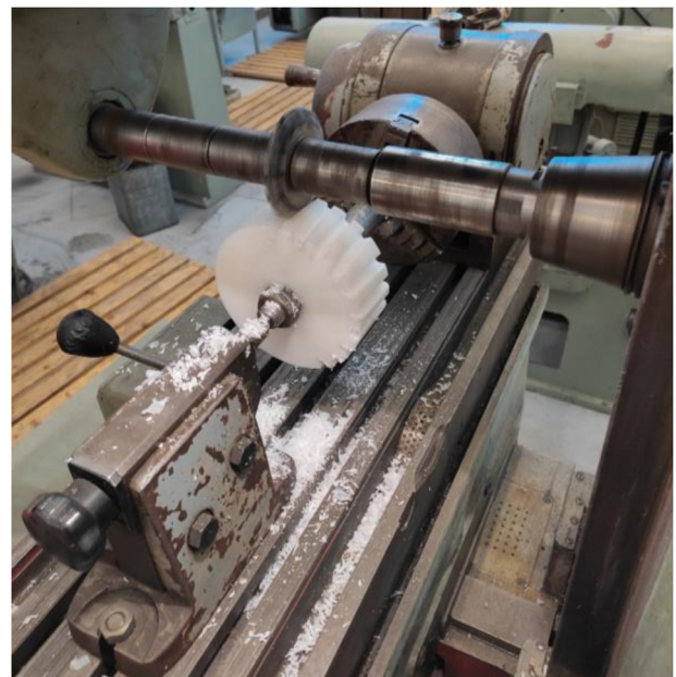
Fig. 9. Spur gear manufacturing by a CNC milling machine
