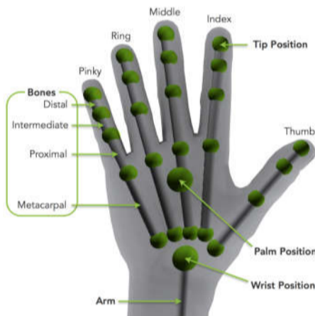
Fig. 3. Leap Motion's hand representation (adapted from http://blog.leapmotion.com/getting-started-leap-motion-sdk/ )
