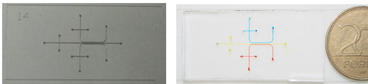
Fig. 1. A mold for the preparation microfluidic chip containing three identical channel system (left), a microchip sealed onto a glass slide and the channels filled with different color dyes (right).
