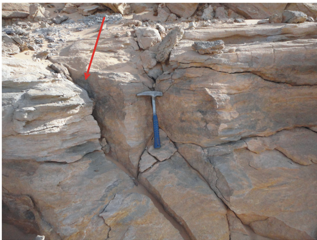
Fig. 5. Vertical, oblique, and horizontal open joints, indicated by red arrows. These discontinuities are filled with loose sand, as seen in Profile 2
