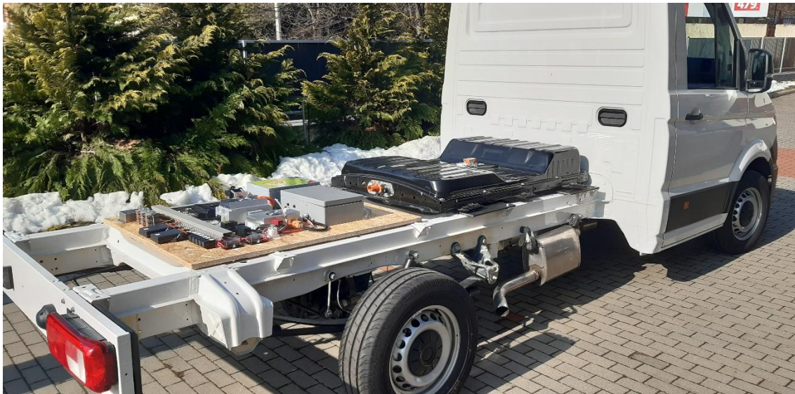
Figure 6. The build-up of the vehicle after the conversion
