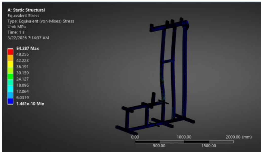
Figure 45: equivalent Stress analysis result
