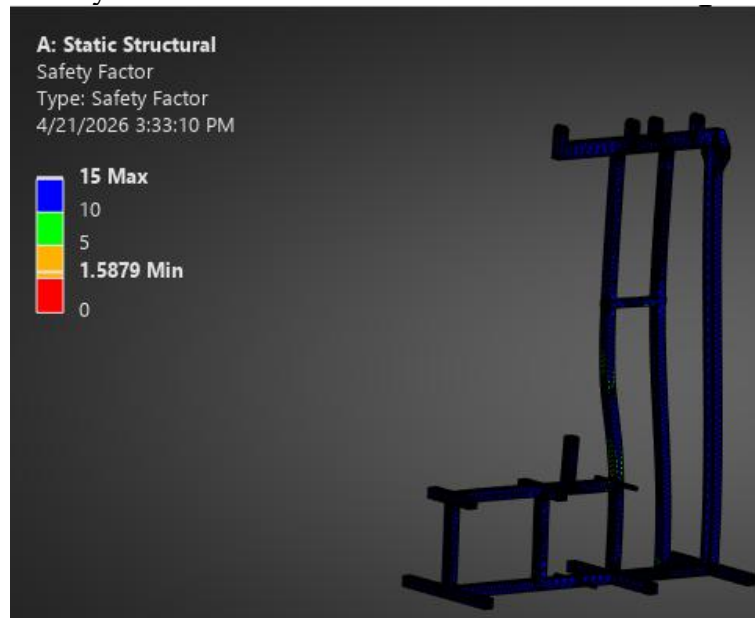
Figure 48: Factor of safety for the modified diagram
