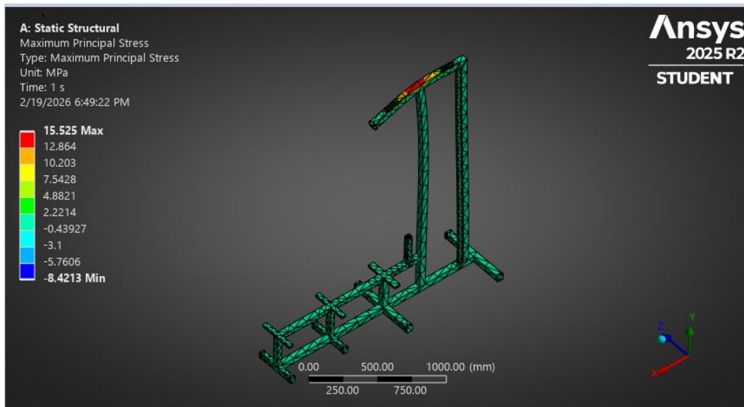
Figure 31: maximum Principal Stress analysis result
