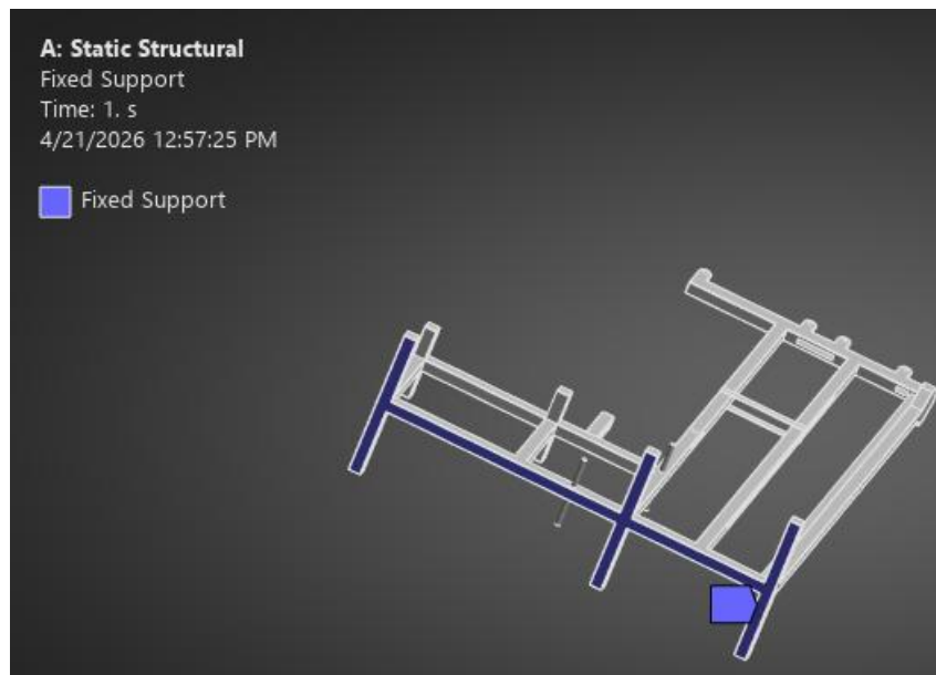
Figure 41: Frame fixed at the bottom part of the frame
