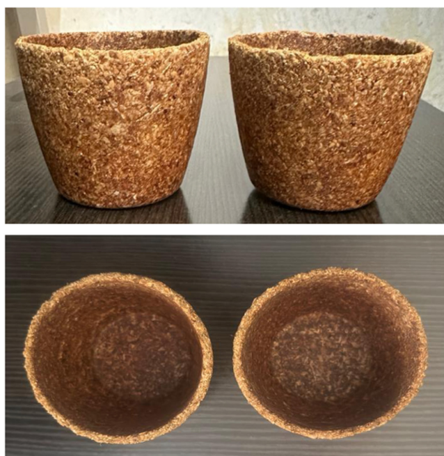
Figure 3. Developed biodegradable cups, front view and top view.
