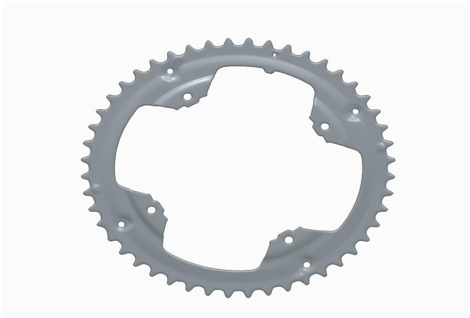
Figure 27: Large Gear CAD Model ( Worn )
