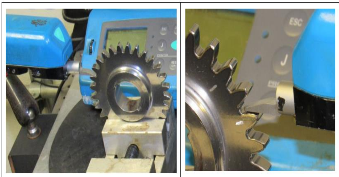
Figure 39: Profilometer ( “Shop Floor” Model ) [16]
