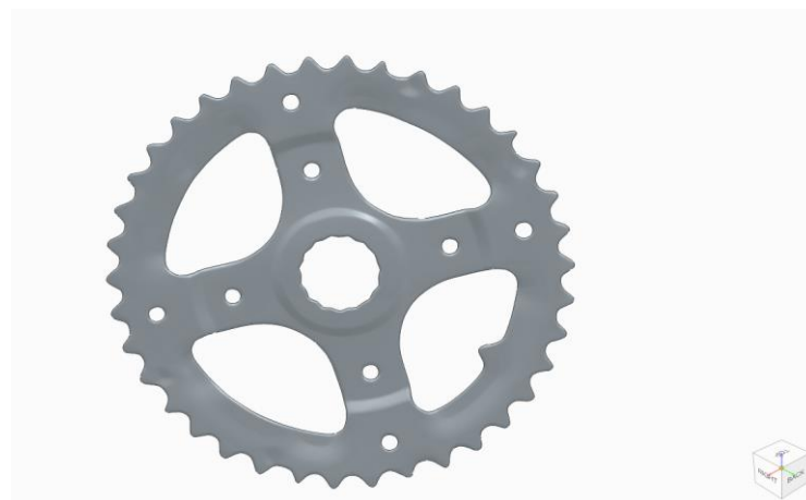
Figure 26: Medium Gear CAD Model ( Worn )
