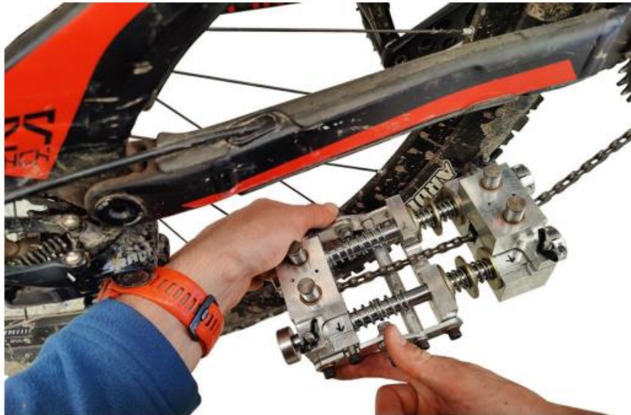
Figure 38: Chain wear checker in-situ operation [15]
