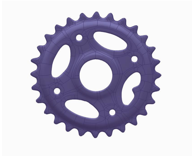
Figure 25: Small Gear CAD Model ( Worn )
