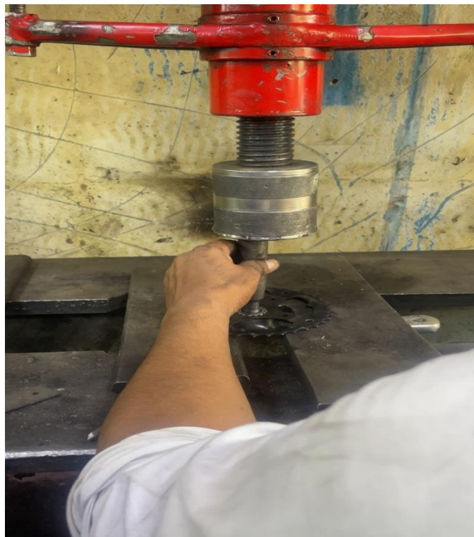
Figure 19: Crank-arm Removal Using Hydraulic Press Machine
