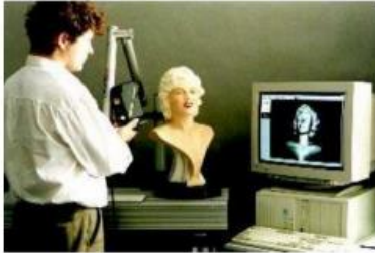
Figure 7: Manually Operated and Strip 3D Scanner [4]
