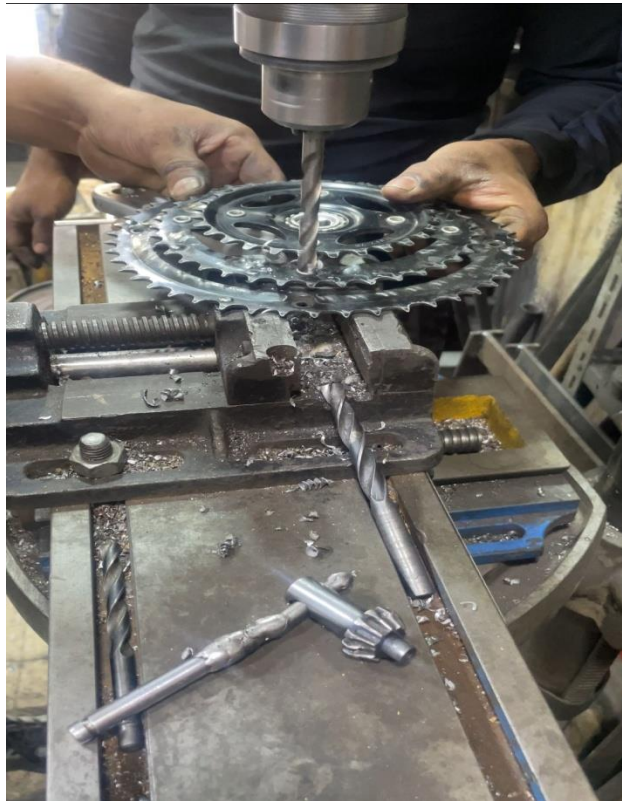
Figure 17: Rivet Removal Process Using Drill Press
