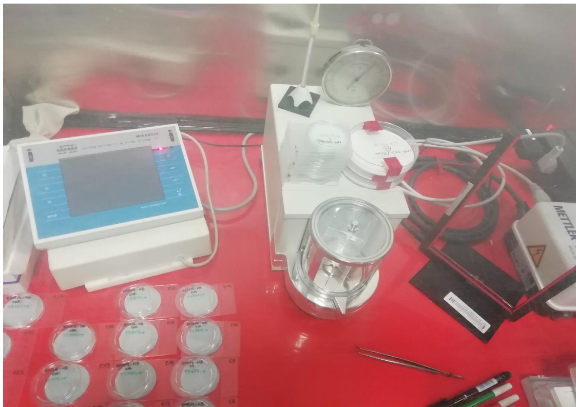
Figure 2.11 the Radwag microbalance with filters in petri slides under conditioning, and the ionisator (right).
