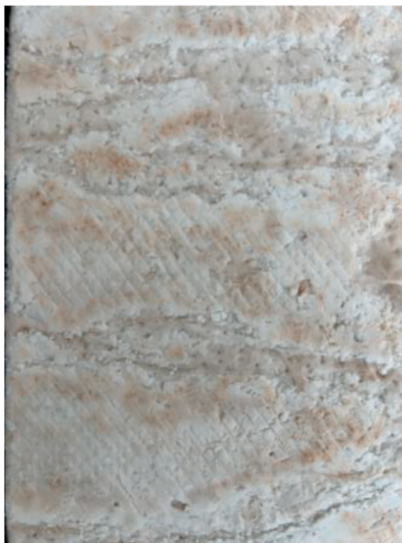
Fig. 7a. Surface photo of the sample annealed at 250 °C for 1 day.
