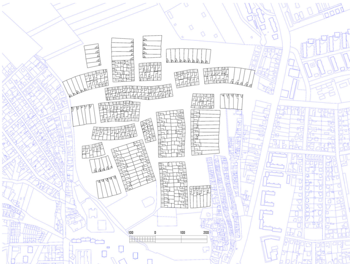
Figure 44. Fourth increment of the growth, top view. Blue: existing plots and buildings; black: new (generated) plots and buildings. Source: author's work.
