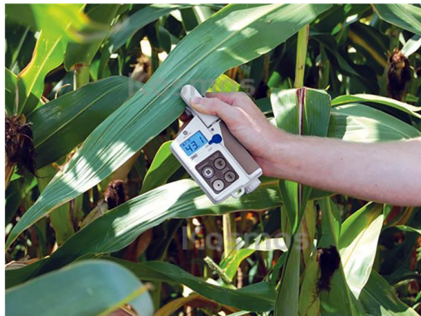
Figure 4 : SPAD-502 relative chlorophyll content measuring instrument
