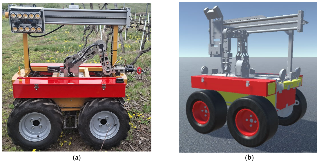
Figure 2. (a) The physical robot; (b) the digital twin.
