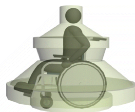
3.12. The maximum diameter of turning is at the height of the foot-rest
