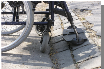
4.2. The footrest may impinge the ramp
