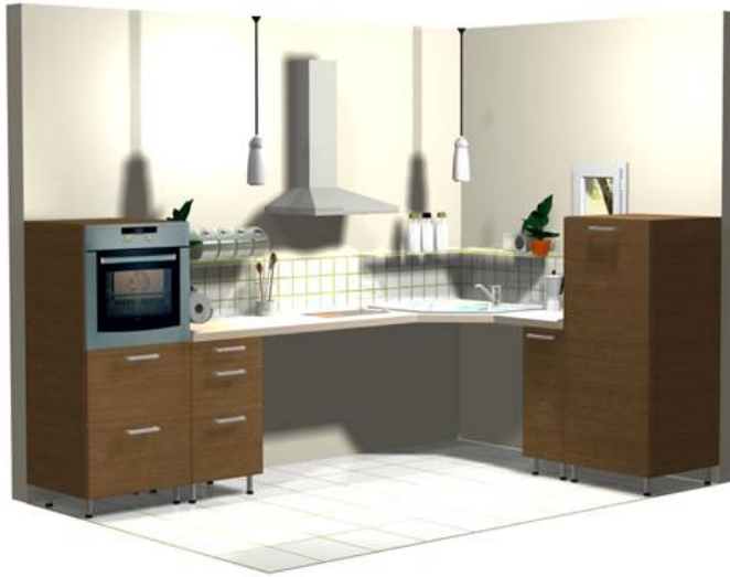
5.15. Knee free counter is to be provided to facilitate the manipulation on the worktop
