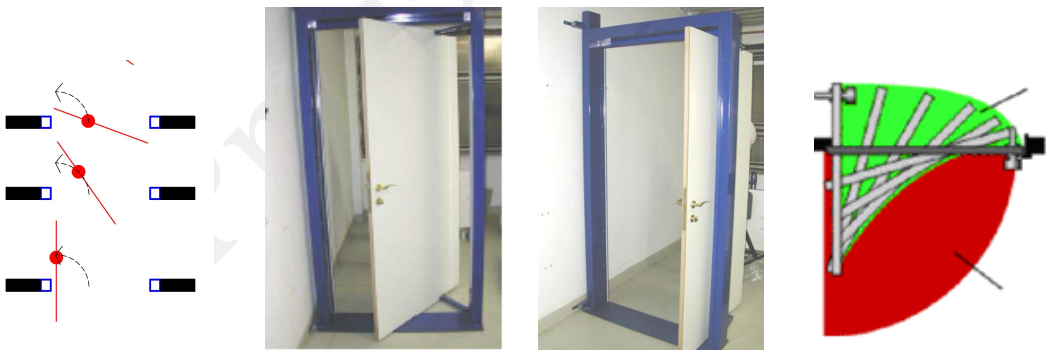
3.18. Hinged pivot door (the photos are from an exhibition, thus the door is not built-in
