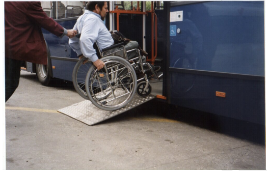
11.8. Steep collapsible ramp does not facilitate the safe and self-sufficient use of bus.
