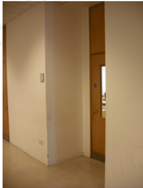
7.7. Doors – especially when suddenly opened – disturb the traffic along the corridor. Bays at doors eliminate this problem.
