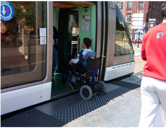
11.6. Marking of doors on the platform accelerates the traffic
