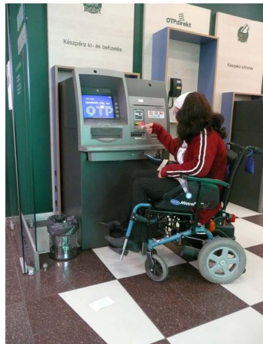
7.9. The operative parts of the machines that must be reached should not be higher than 120 cm.
