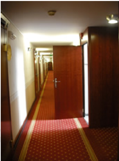
7.7. Doors – especially when suddenly opened – disturb the traffic along the corridor. Bays at doors eliminate this problem.
