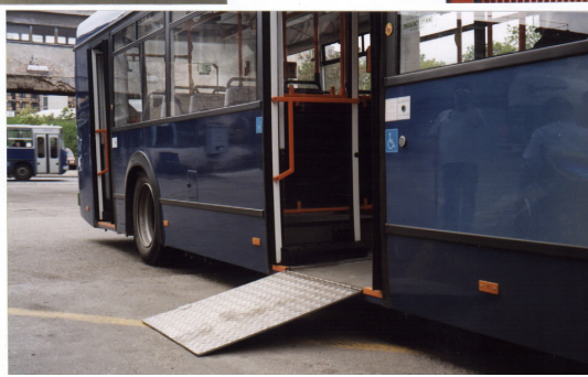
11.8. Steep collapsible ramp does not facilitate the safe and self-sufficient use of bus.
