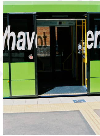
11.6. Marking of doors on the platform accelerates the traffic
