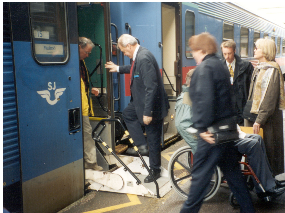
11.15. Platform lift under the floor of the carriage
