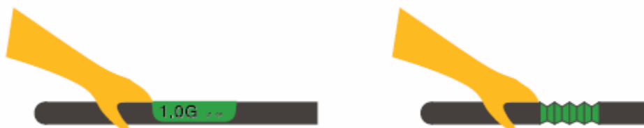
9.7. Escape route can be marked on handrails, too
