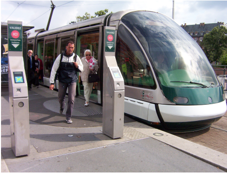
11.4. Stop of low floor tram with accessible information column and ticketing machine
