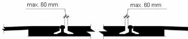
10.18. The acceptable gap along rails
