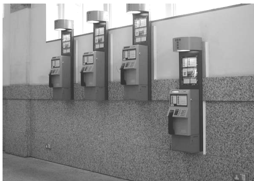
7.10. Group of public phones – one of them can be reached from wheelchair
