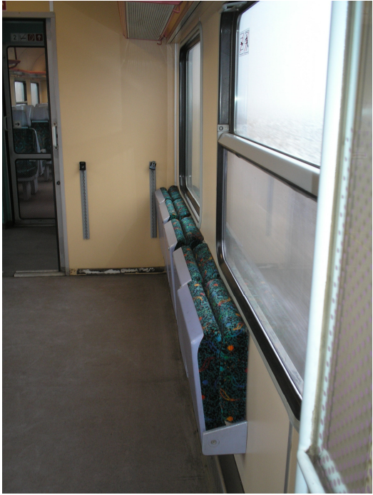
11.18. Collapsible seats provide free place
