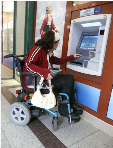
7.9. The operative parts of the machines that must be reached should not be higher than 120 cm.
