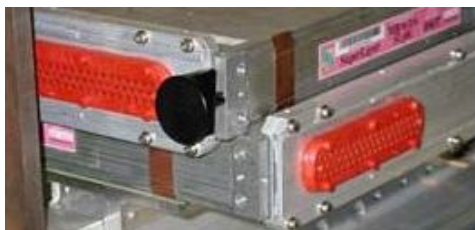
Figure 8.3. Part of the barrel muon chamber equipped with a photogrammetry test-target.
