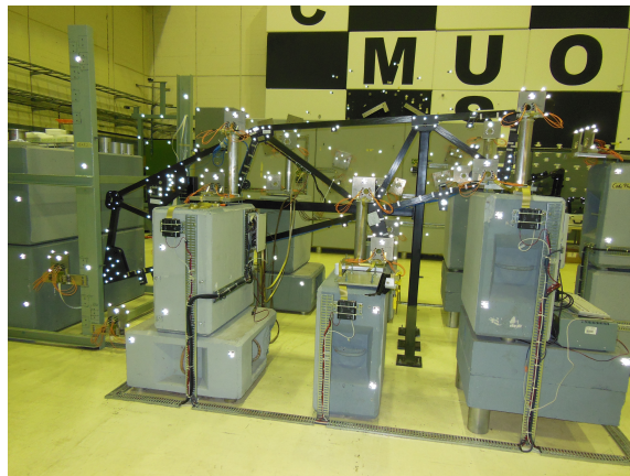
Figure B.4. The illuminated retroreflective targets during the MAB calibration.
