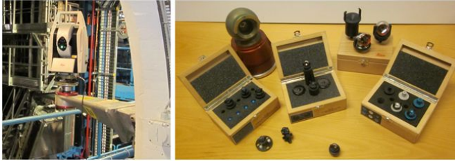
Figure B.1. The LEICA AT401 Laser Tracker in work in an experimental hall (left) and different targets and adaptors (right).
