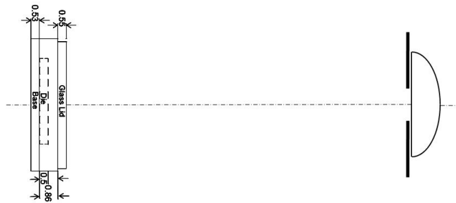
Figure 6.5. The inner structure of the camera-box.
