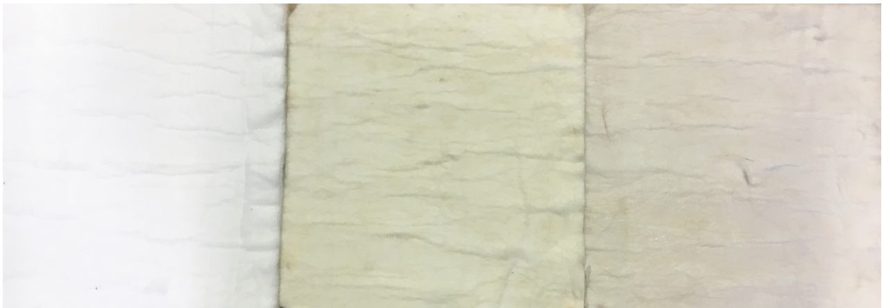
Figure 12. The photographs of the un-annealed sample (left), the annealed sample at 70 °C for 6 weeks (middle) and the annealed sample at 210 °C for 1 day (right)
