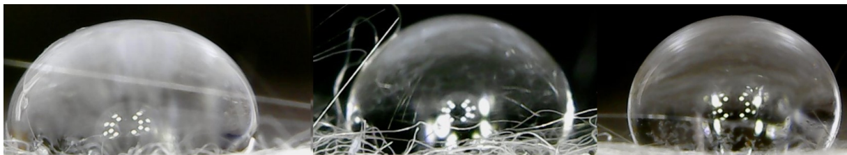
Figure 14.: The result of the hydrophobicity tests of the samples, from left to right: the as-received, annealed at 70 °C for 42 days, annealed at 210 °C for 1 day
