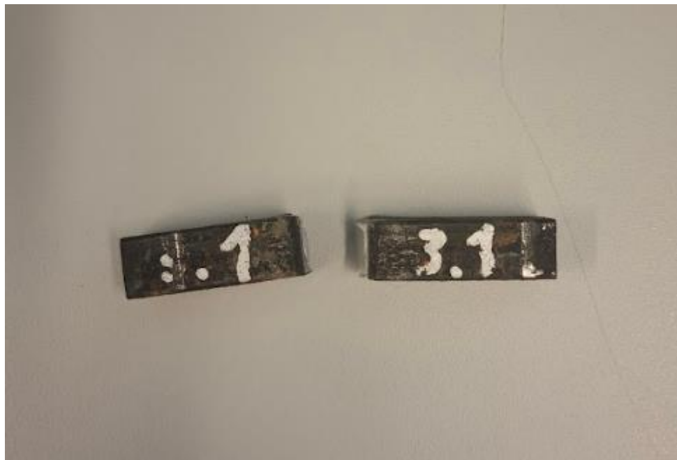
Figure 4.6 Sample 3.1 after the Impact
