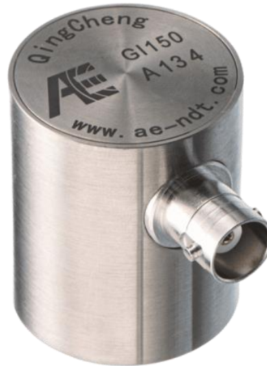
Figure 2.6 Acoustic emission sensor [12]
