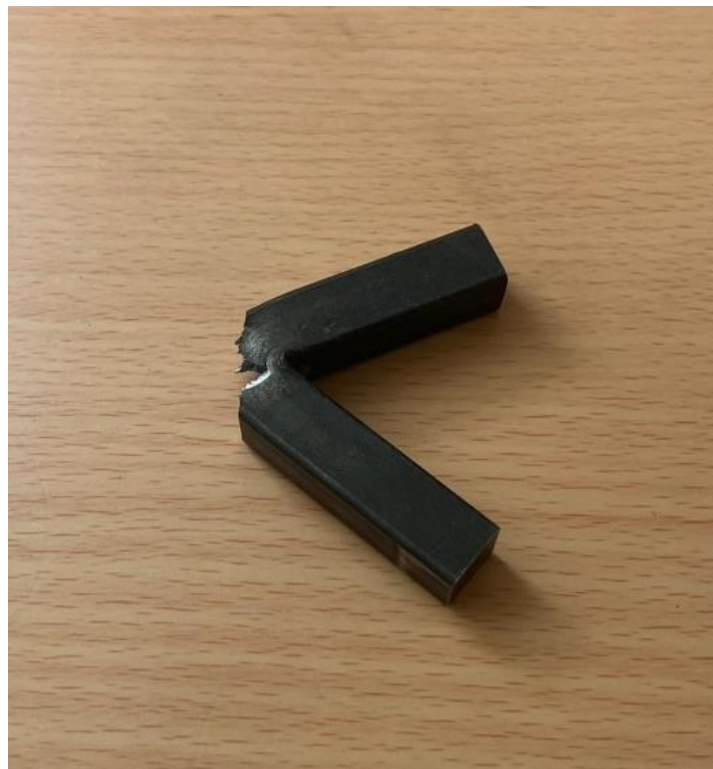
Figure 3.5 Specimen after impact test
