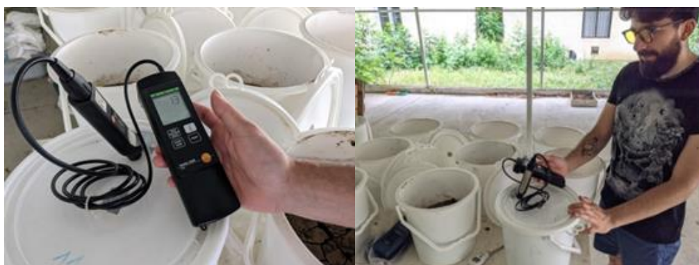
Figure 4. Measuring with Testo 535 infrared gas analyser
