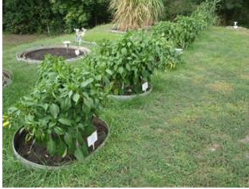
Figure 2. Simple drainage lysimeters dedicated to the study of secondary salinization at the Research Institute of Karcag in June, 2019
