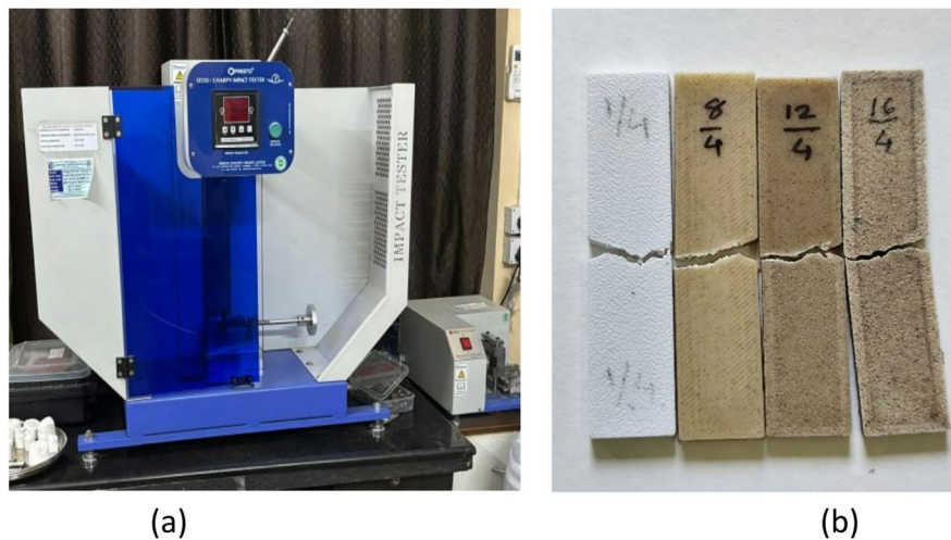
Fig. 7 (a) Impact tester, (b) Impact tested specimen
