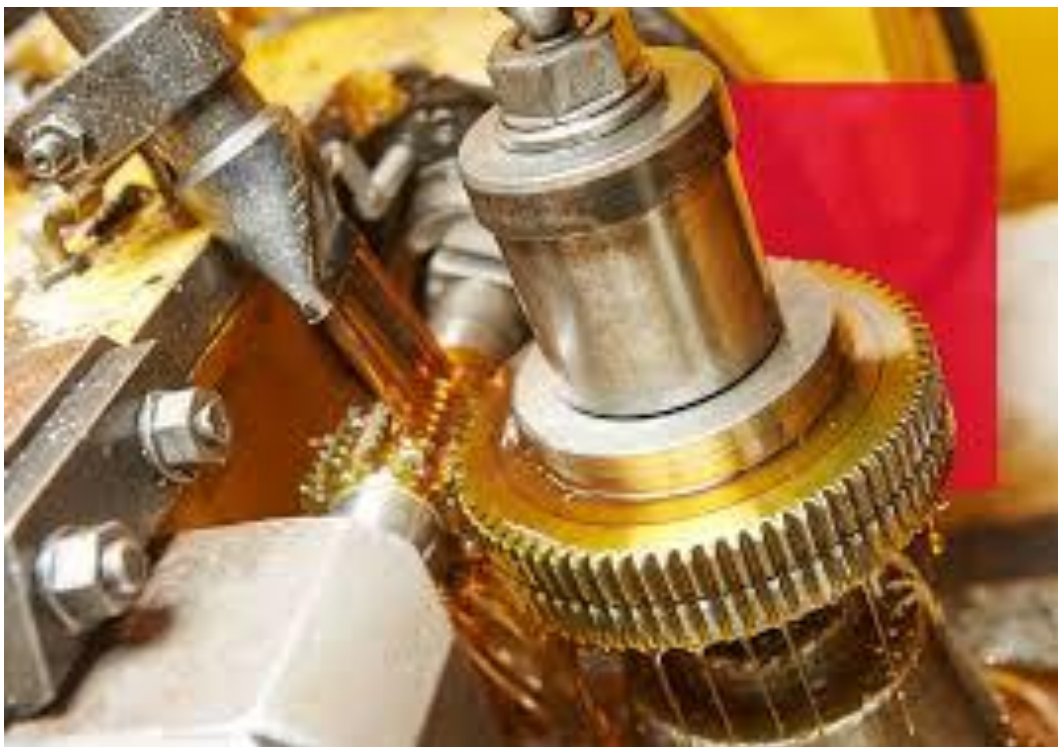
Figure 1.2 Gear Hobbing Operation [7].
