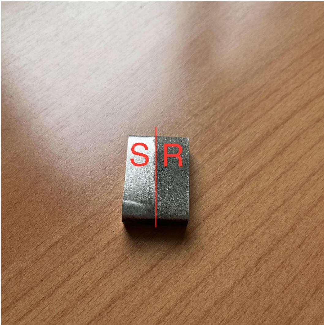
Figure 4.6 – Smooth and rough areas of the specimen
