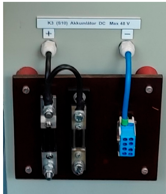
Figure 6. Shunt resistors for measuring the electric current intensity.
