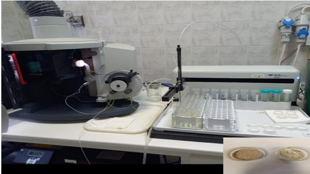
Figure 6. The elemental composition detection in various grain fractions by using the ICP-OES technique
