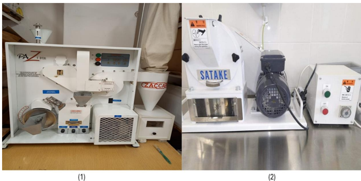
Figure 9. The utilized huskers (1) Zaccaria No. 1. testing rice mill for 60 (S), Institute of Research, Karcag. (2) Satake husker for the husking technique, Lab of Food Science and Technology.
