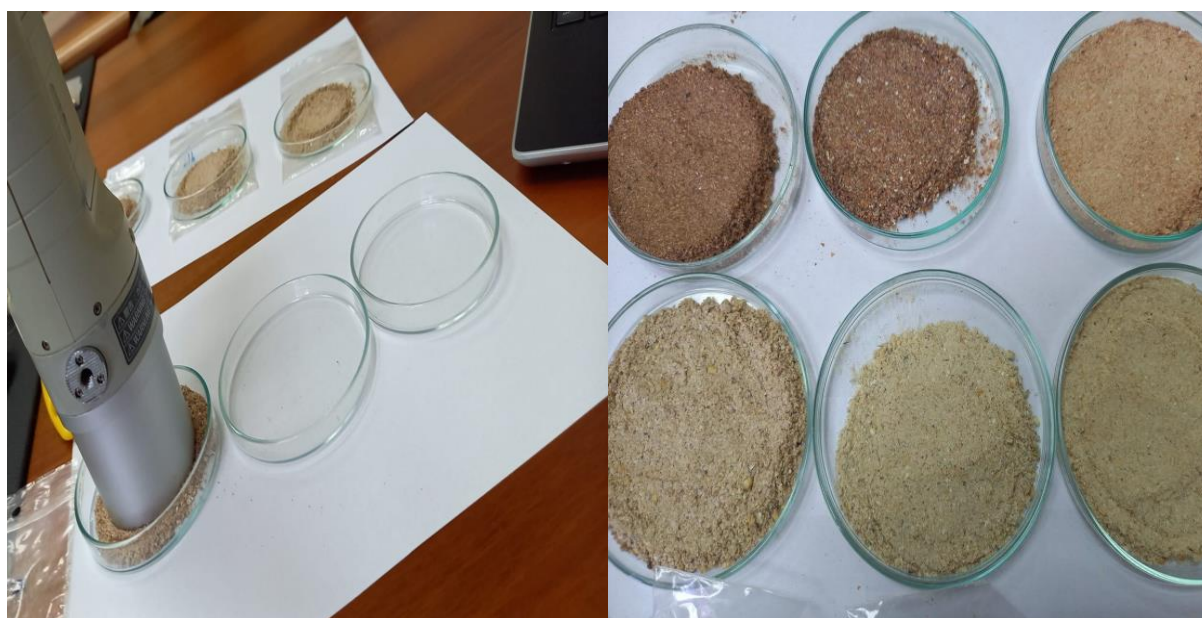
Figure 10. Measurement of the colour profile of the respective grain varieties by utilization of CR-410 Konica Minolta Camera
