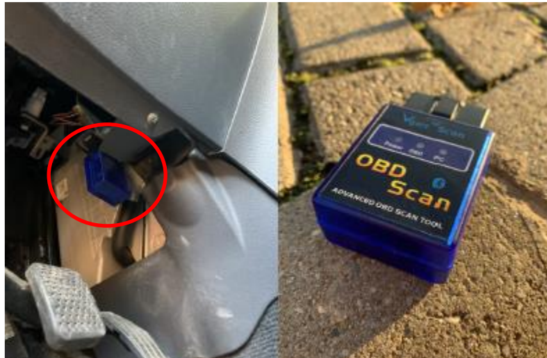
Figure 2. The device used for the measurements, ELM327 Vgate Scan Advanced OBD2
