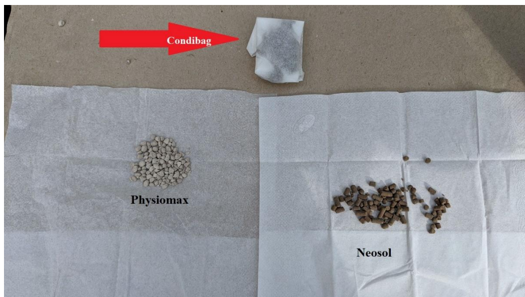
Figure 52. Preparing a condibag for micro soil conditioning
