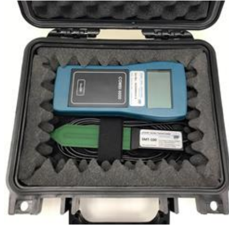
Figure 9. SMT-100 soil moisture probe (Source: I2)
