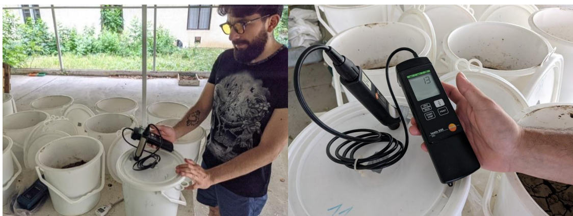
Figure 16. Measuring with Testo 535 infrared gas analyser
