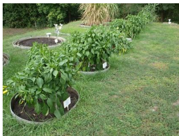
Figure 6. Simple drainage lysimeters dedicated to the study of secondary salinization at the Research Institute of Karcag in June, 2019
