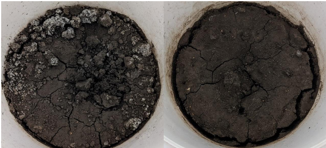
Figure 49. The soil surfaces irrigated with tap water (left) and deionized water (right) in the pot experiment (Karcag, 2022)
