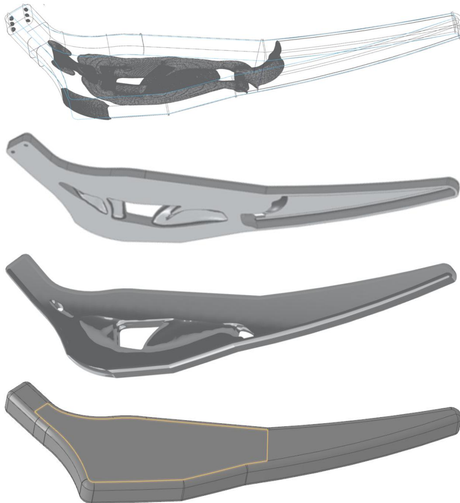
Figures 2.22., 2.23., 2.24., 2.25. & 2.26. Internal Channels (wireframe, sliced) in 25 % Weight in the selected face of the Original Hip Implant Model
