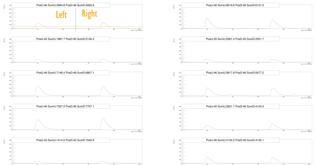
Figure 8. For 10 saved inputs, the two opposite SiPM signals are shown and the triggering condition is indicated by the orange line.
