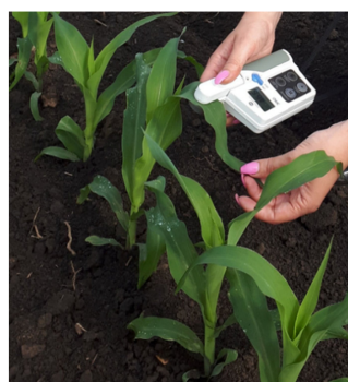
Figure A1. Illustration of the use of the handheld SPAD measurement device in the maize population.
