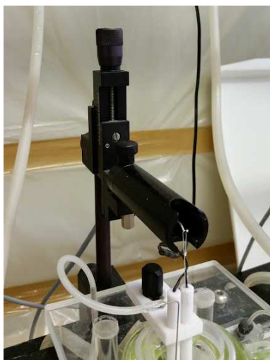
Fig. 11. The transducer used for the detection of the amplitude of isometric twitches
