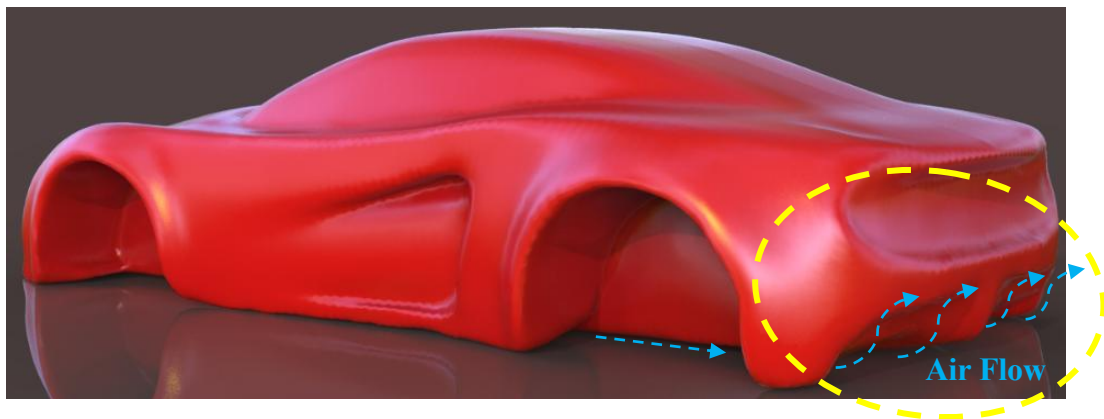
Figure 2.9 Air flow through the bottom and rear diffuser of the concept car.
