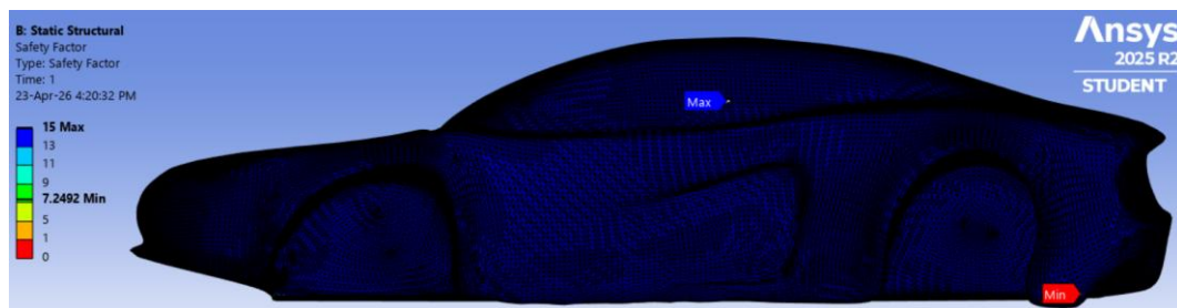
Figure 3.38 Safety Factor, Tensile Yield Per Material at 3.2e+003 (Auto Scale).
