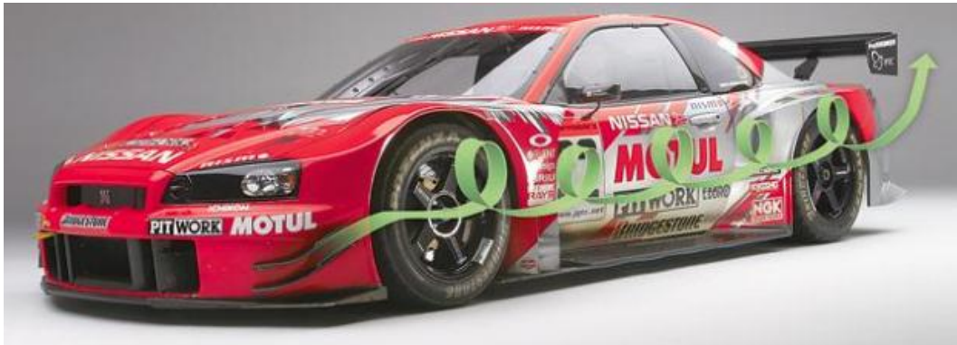
Figure 1.7 Vortices created by the Canards. [11]
