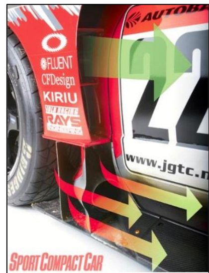
Figure 1.10 Airflow pattern through the Side skirts channels. [11]
