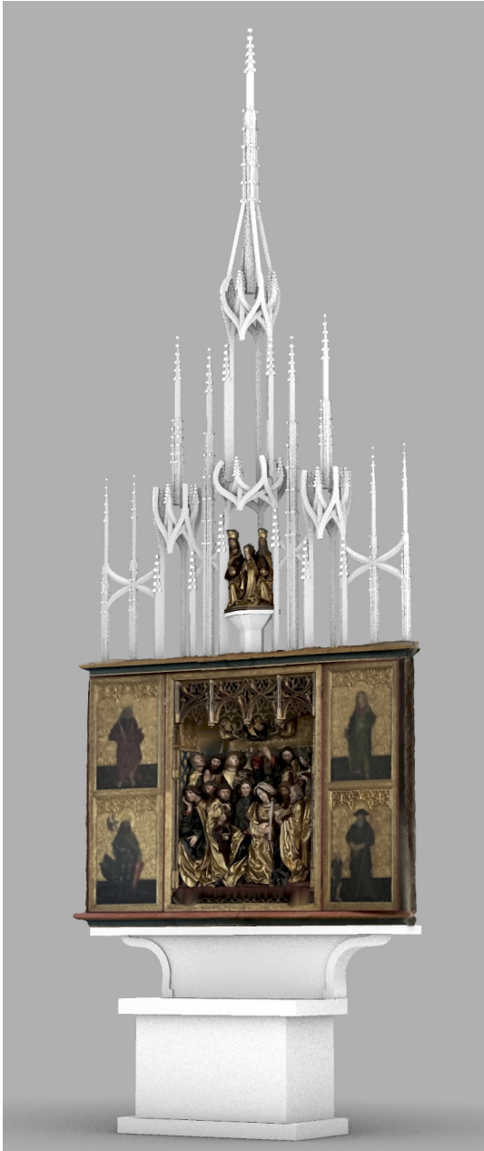
Figure 15: Algorithmically generated model of the destroyed crown of the Altar of the Death of Mary, with the photo-scanned 3D model of the altar. The algorithm is based on the crown of the surviving Altar of the Coronation of Mary, and the parameter values are based on the nineteenth-century survey drawing. Source: Author's work.
