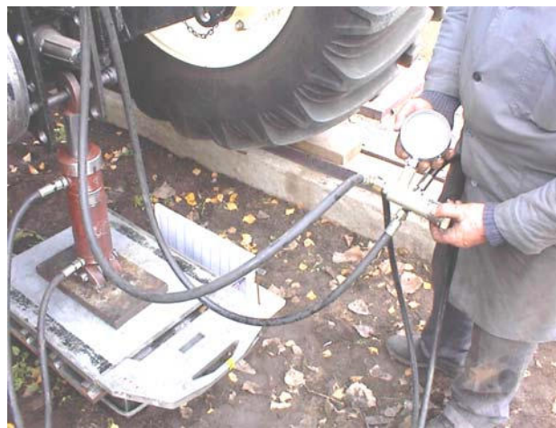
Fig. 2. Penetration of the pushing tools into the soil
